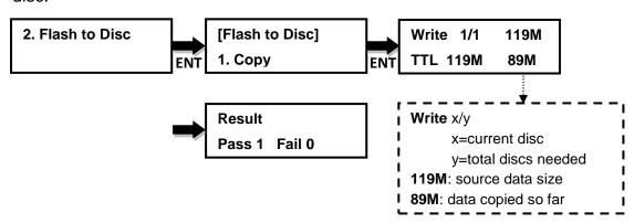
**b.** Second example: A USB drive with 1115MB data content is copied onto three CD discs.
