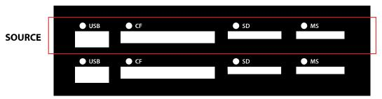
Use only one of the USB, CF, SD or MS slots on the top row as the source and one of the slots at the 2nd row below as target for duplication. Do not plug in 2 or more USB and memory cards as source or target at the same time.
