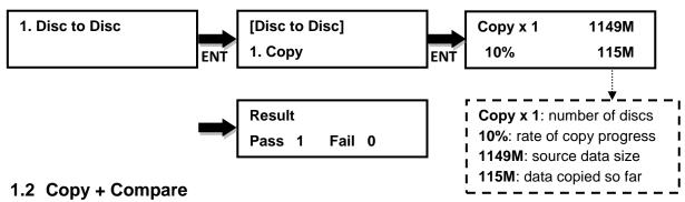
This function performs a copy first, then automatically compares the data between source and copied discs to confirm that an exact clone has been created.
