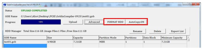
■ Format the internal SSD in the PCIE duplicator.
