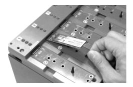
Step 4: Place M.2 SSD securely all the way down and release the rubber
