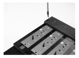
Caution Please use extreme caution while using a screwdriver to remove the screws as it can easily slip and damage the surrounding area.
