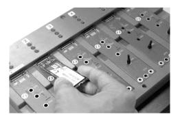
Step 2: Insert M.2 SSD at an angle to connecting port.
