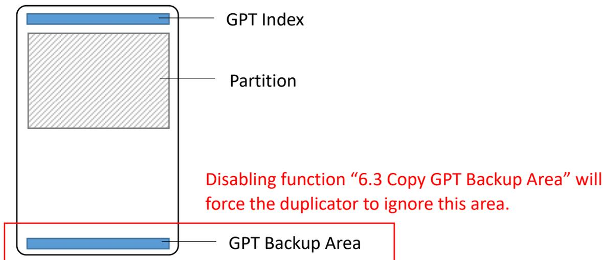
**Caution** If function is disabled, the target HDD will reconstruct the GPT Backup Area by Windows system. It may require the HDD to restart to work.
