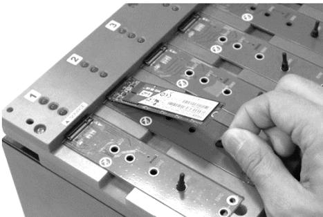
**Step 4: Place M.2 SSD securely all the way down and release the rubber standoff.**
