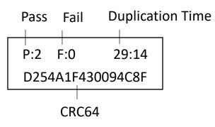
Note CRC64: During duplication, each port will simultaneously record written message and compare CRC64 between source and targets. The result will show light in red(fail) or green(pass).
