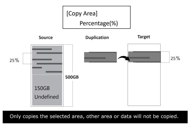
Caution It is recommended to execute Compare after Copy to confirm the accuracy. It is recommended to copy data by function "3.Copy+Compare".
